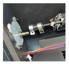
Disconnect the motor , from the rod
