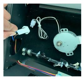
Pull out the wiring and unplug the motor
