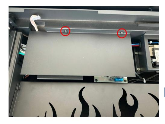
Unscrew the screws to take off the PCB board protection cover.
