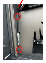
Unscrew 2 screws on each on left and right hand side to remove the flame stencil.
