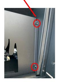
**Step 2** The flame light is located at the back of the flame stencil. Now you can replace it with a new flame light.
