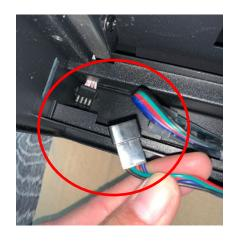
Unbuckle tray light to disconnect the tray light assembly from the fireplace, remove and replace.
