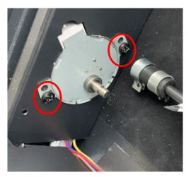
Unscrew the screws to remove the motor
