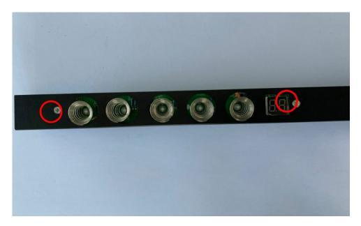
Unscrew the screws to remove the touch panel to replace it with a new one
