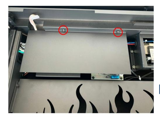
Remove the screws to take off the PCB board protection cover.
